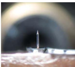
Figure 13 : Bent etched fiber perpendicular to tip
