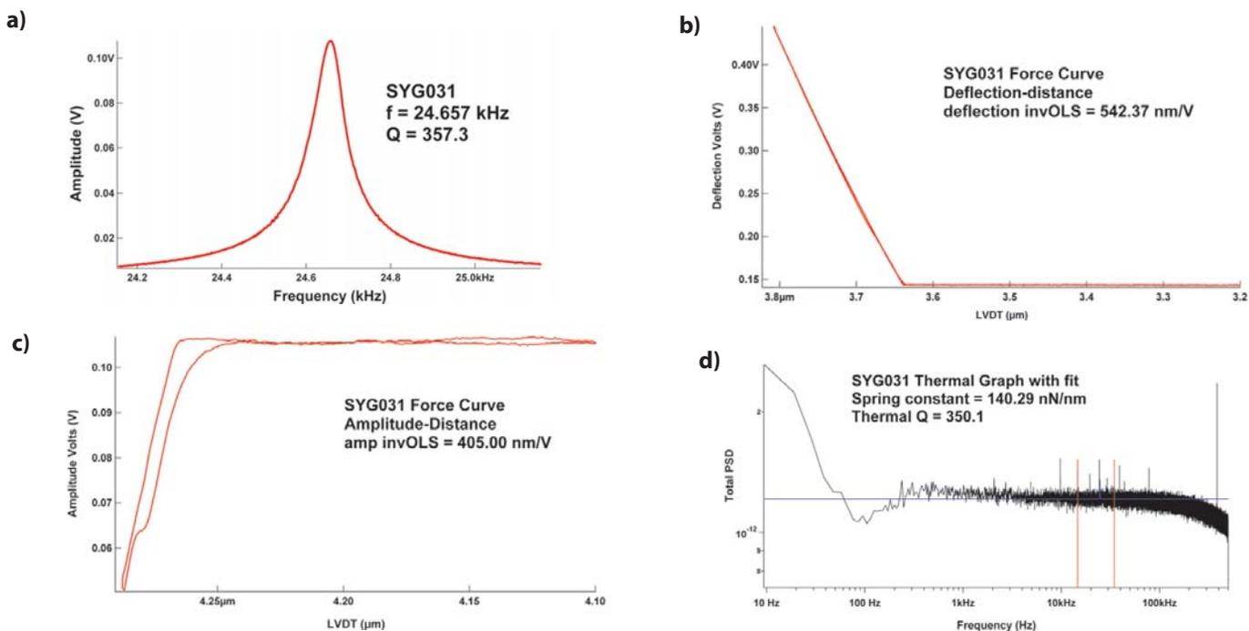
**Figure 19:** Graphs used in the measurement of the spring constant of tip (meniscus - selective etch) using the AFM: a) The cantilever tune, b) deflection-distance force curve, c) amplitude-distance force curve and d) thermal graph.
