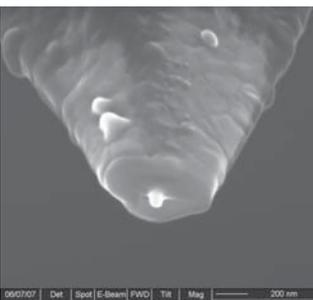
Figure 16 : Antenna on tube etched tip (SEM)
