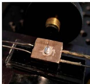
Figure 12 : Silver epoxy curing on heater plate
