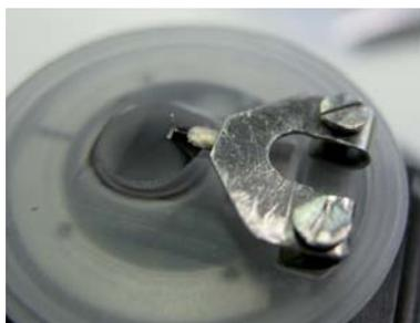
**Figure 20** : New clip for the AFM tip holder
