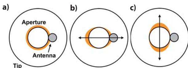
**Figure 3:** Polarization of light with respect to the aperture-antenna alignment (as indicated by the arrow), where a) no polarization, b) polarization aligned, c) polarization misaligned. The signal is greatest in b) where the polarization is aligned, and lowest in c) where it is completely misaligned, whereas in a) the distribution is even.
