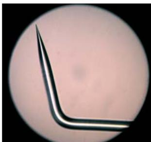
Figure 11 : Bent fiber, 105.6° (10x magnification)
