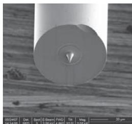
Figure 6 : Selectively etched tip (SEM)
