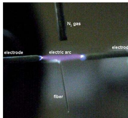
Figure 10 : Electric arc bending of optical fiber
