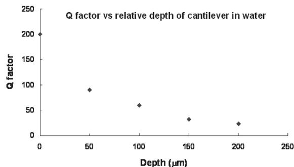
**Figure 23** : Q factor vs. relative submerged depth of cantilever in water. The depth is measured from the point where the tip first touches water, so the first measurement in water is at 0  $\mu\text{m}$  with a Q of 200.
