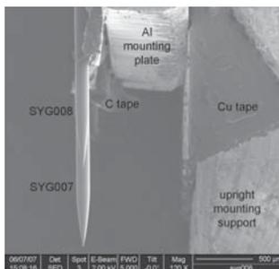
Figure 15 : FIB setup for upright fibers (SEM)
