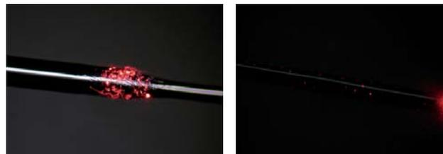
Figure 9 : Photographs of a tip coupled to a laser as viewed from under an optical microscope. We observe a) imperfections in the coating due to uneven etching at the meniscus of a thinned fiber and b) small pinholes along the taper of the fiber from dust particles in the solutions and a large pinhole at the tip.
