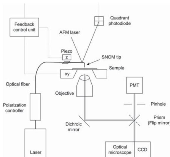
**Figure 4:** Transmission mode SNOM setup schematic
