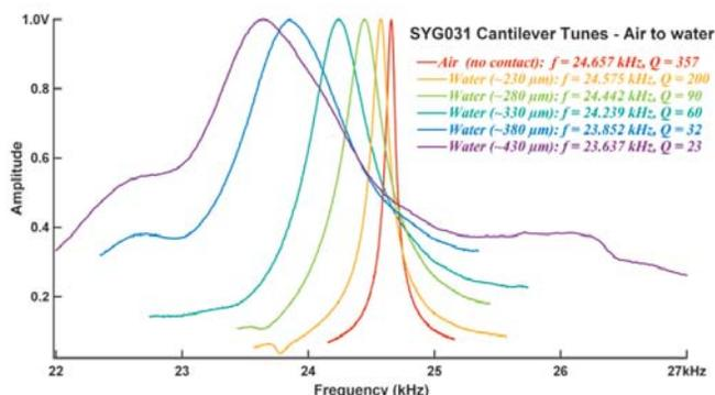
**Figure 22** : Resonance curves of a tip (meniscus – selective etch) as it is lowered into the liquid from air. The curves have been normalized for the purpose of comparison. The original amplitude value is not relevant since it depends on the drive amplitude.
