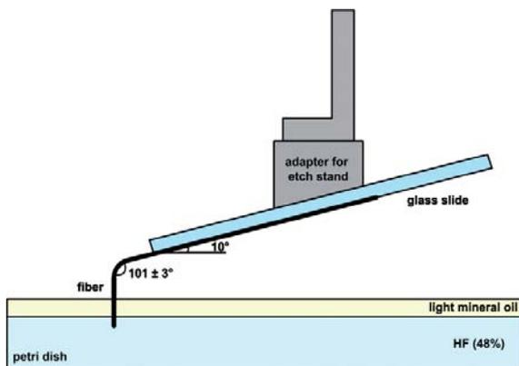
Figure 8 : Setup for etching bent fibers.
