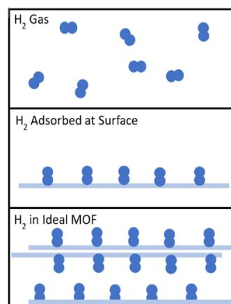
Figure 1. Schematic showing principle behind adsorptive H<sub>2</sub> storage. While it is counterintuitive that more H<sub>2</sub> can be fit into a space also containing an MOF, the lowering of pressure through adsorption allows a significant increase in g H<sub>2</sub>/L.
