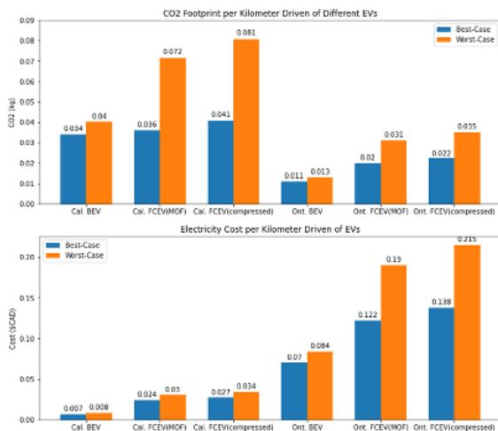
Figure 10. Results of refueling model. FCEV using 700 bar compressed system was added for comparison, by scaling MOF-FCEV values by factor shown in Table 3. Compressed-H<sub>2</sub> FCEV values are likely underestimated due to the model being tailored towards MOF-FCEVs.
