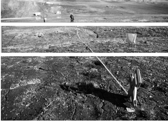
Fig. 5. The white box shows the local depression that formed on the NW side of the runway near T4, as a response to the disturbed subsurface water flow.
