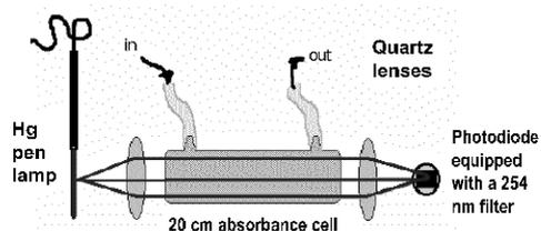
Figure 3. Schematic of the atomic absorption spectrometer (AAS)
