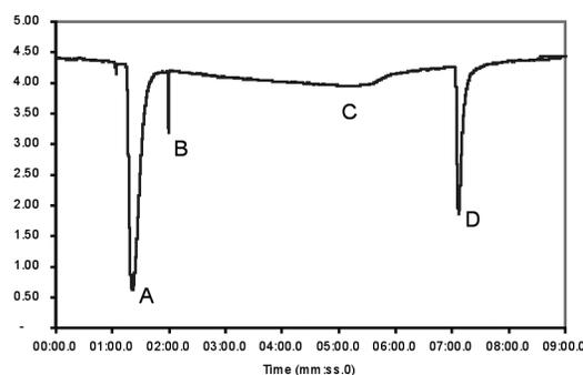
Figure 4. AA spectrum of a single hair strand (10 pt moving avg)
