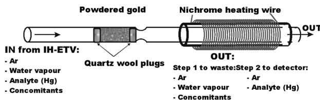
Figure 2. Schematic of the gold amalgamation (GA) trap
