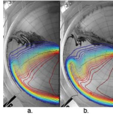
**Figure 5.** Image a shows the numerical model (colored lines) superimposed over data from an experimental run at  $Q=10\text{cm}^3/\text{s}$  and  $\delta=0.0025$ . Image b shows the same for  $Q=20\text{cm}^3/\text{s}$  and  $\delta=0.025$ .
