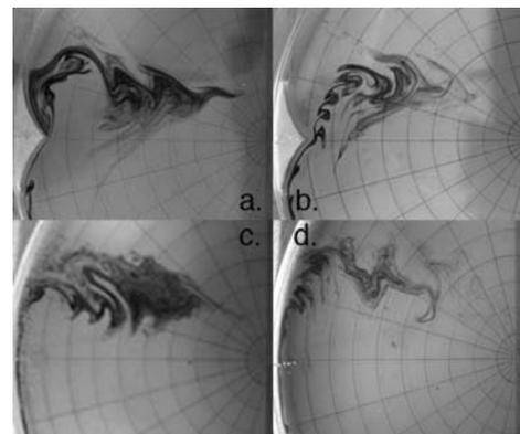
**Figure 6.** Image a shows results from an experiment at  $Q=10\text{cm}^3/\text{s}$  and  $\delta=0.0025$  with the cape insert. Image b shows results at  $Q=10\text{cm}^3/\text{s}$  and  $\delta=0.025$  with the cape insert. Image c shows results of the same setup as in a, without the cape. Image d shows results of the same setup as in b, without the cape.
